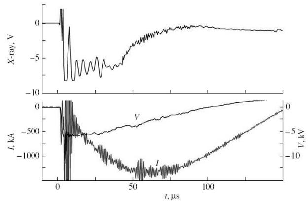
Fig. 2: Typical oscillograms of current, voltage and x-ray signal
