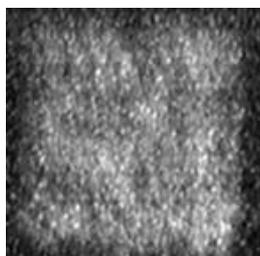
Fig. 1: Radiography image of discharge gap at 20 $\mu$ s after initiating discharge with current amplitude 600kA
