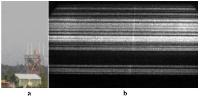
Fig. 2. a – A view of the tower in the same scale as it is seen by the K004M camera; b - A sweep (full duration is  $10.65 \mu\text{s}$ ) of the images of an exploded rocket wire and a grounding wire of the unit of launching tubes. A vertical size of a field of view is 37.5 m.
