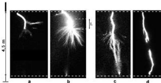
negative discharge development in a rod-rod gap was obtained (Fig. 1). The frames demonstrate, in succession, a) an initial corona, b) a leader stage (L is leader step) with a powerful flash of streamers, c) a pass of the process to a through phase at the expense of positive and negative streamer zones merge and, finally, d) a meeting of the channels of negative downward and positive upward leaders.
