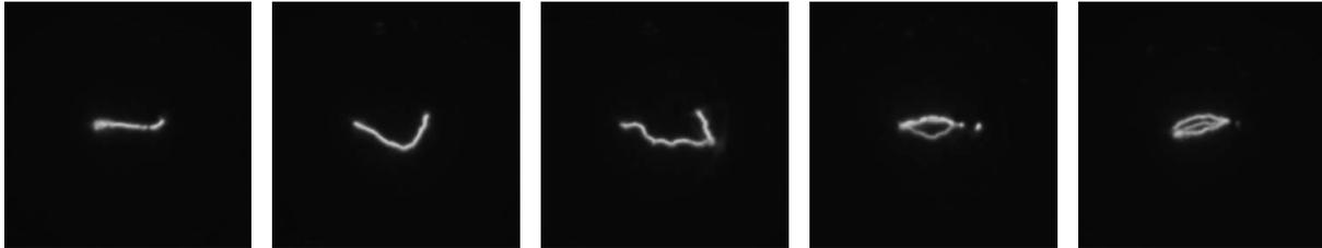
Fig. 9. Other different realization of discharge channel formation. Parameters of experiments corresponds to fig.6. The exposition – 10 ns. And the moment of exposition synchronizes to moment of maximum current at the first half-wave. High-speed camera – NanoGate-1. Spectral range of filming is 600-700 nm.
